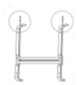
Unscrew the two screws holding the wall mounting bracket to the back of the body, and keep in a safe place to allow the option of wall mounting in the future.
