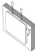
Tighten the two screws on the top of the bracket, ensuring the unit is secure, before connecting the power.
